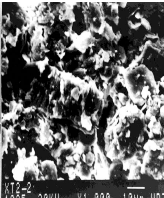
Fig. 14 Micro-texture after water soaked loess, the rounded aggregations disintegrate, parts of them fall in the pores
