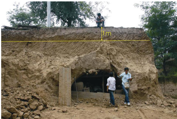
Fig. 17 Ground saturated zone after decades of intermittent rainfall, the observed site is located in Ganquan County, Shaanxi Province
