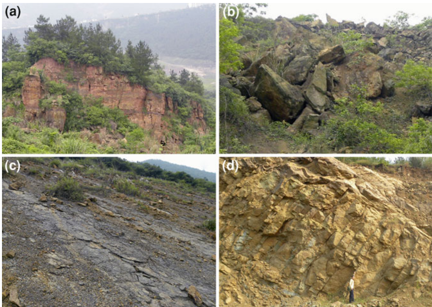
Fig. 8 Photos of a blocky rock mass at the middle-upper part of sliding mass; b disjointed rocky blocks at the upper part of sliding mass; c carbonaceous shale on the main scarp; d bedrock near the main scarp. Locations of these photos are shown in Fig. 4
