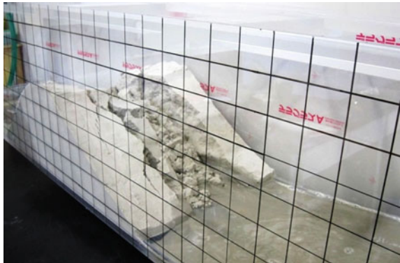
Fig. 21 Temporary breach formation as upstream lake rises steadily due to collapse of dam roof
