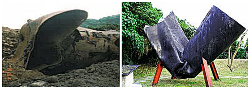
Fig. 6 The distorted 2000 mm steel pipe in Fengyuan ( left ) is now exhibited at the museum of drinking water, Taipei ( right )
