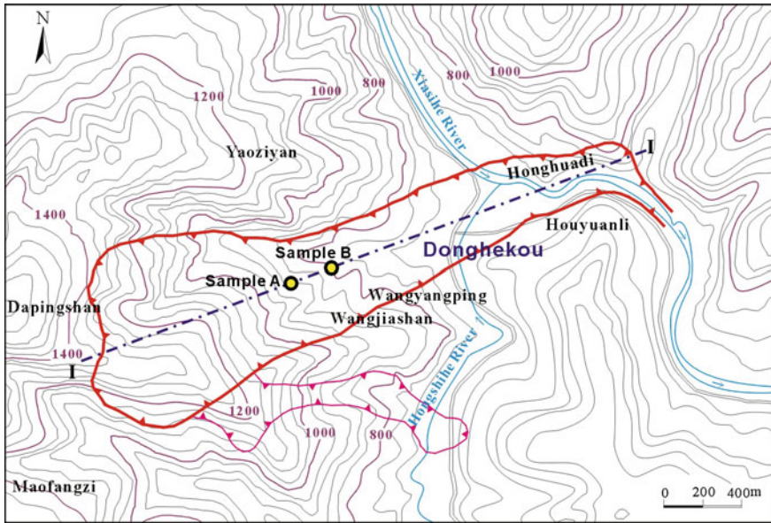
Fig. 7 Topographic map of the Donghekou rockslide—debris flow showing towns, rivers, and areas where samples A and B were taken (landslide boundaries are outlined in lines with triangle marks)
