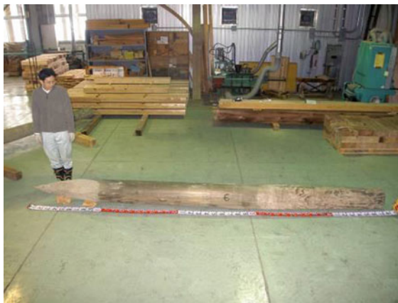
Photo 5 Wood pile retrieved from Kida Bridge
