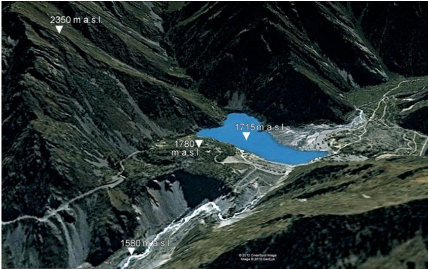
Fig. 5 The Issyk dam and Lake after restoration of the dam. The rockslide headscarp is on the left. Large alluvial fan was formed by debris flow that caused the dam's breach in 1963. 3D Google Earth view
