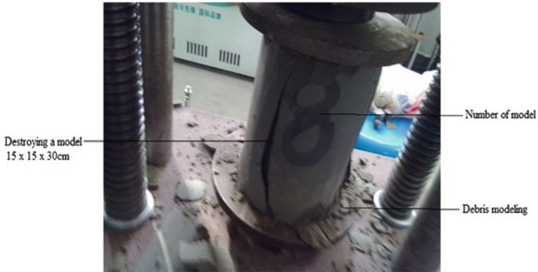
Fig. 4 Typical compression to failure using compression testing machine
