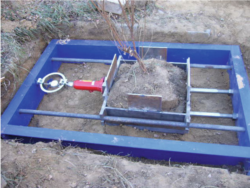
Fig. 18 Photo of the in situ direct shear equipment with a small AF within
