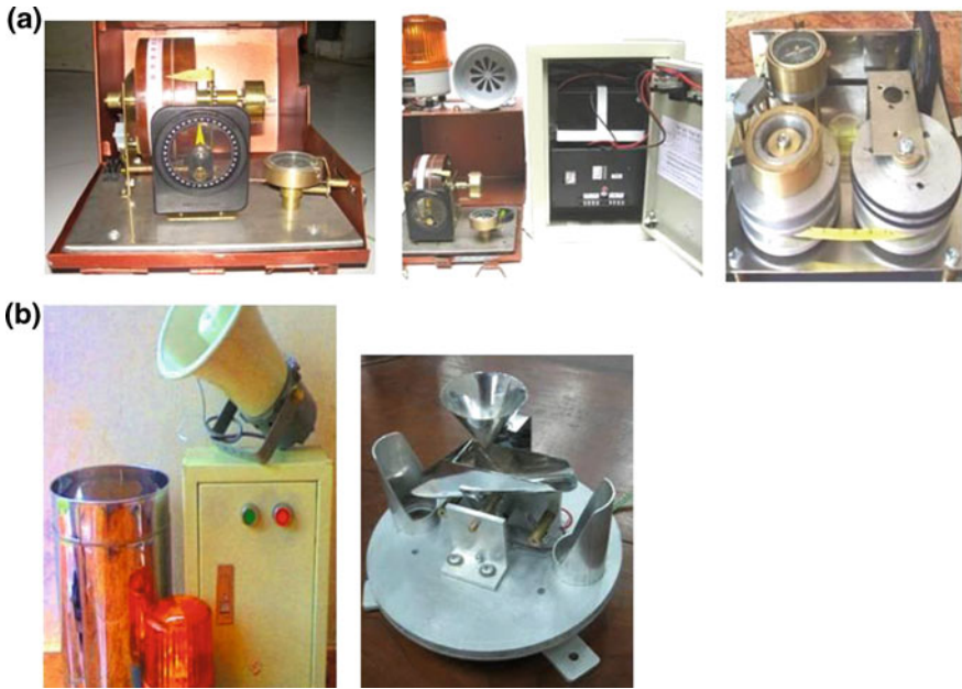
Fig. 3 a Above, the manual extensometer (generation 1 on the left and generation 2 on the right), connected with alarm system in the middle, and b below, the rain gauge with the alarm system (Fathani et al. 2008; Fathani and Karnawati 2009)
