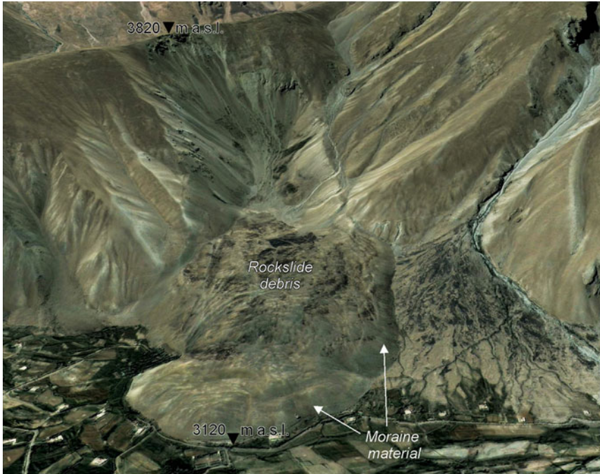
Fig. 11 The Imom rockslide at the left bank of the Gunt River valley. Frontal and flank parts of its body are composed of moraine material resting at the slope base that had been bulldozed by moving rockslide debris. 3D Google Earth view
