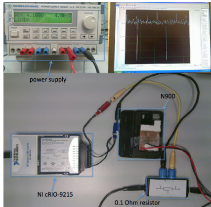
Fig. 2. Experimental setup for measuring power consumption on the Nokia N900
