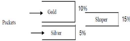
Fig. 6. Create one queue for Gold profile and one queue for Best Effort profile
