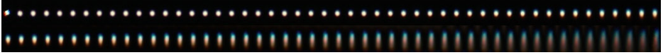
Fig. 4. Measured image quality deterioration of the test chart from the center to the corner. The first line is the dot expansion from 0% to 49% with the step of 1% in radius. The second line is from 50% to 99%. The horizontal is tangential direction while the vertical is radial direction.
