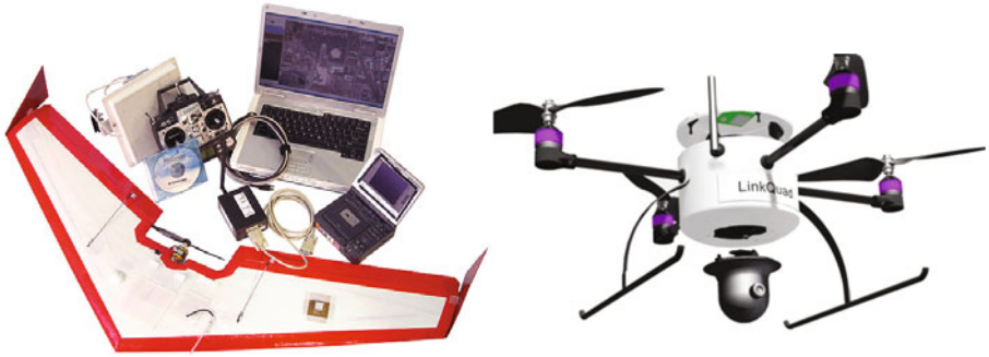
Fig. 4. AgentFly UAV hardware platforms. Left, Procerus fixed-wing aircraft with the development toolkit; Right, LinkQuad vertical take-off and landing quad-rotor aircraft.
