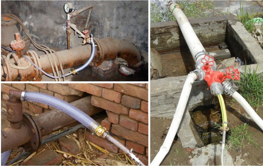
Fig. 2 Connection setups for copper tube sampling from wells. Ideally, a plastic tubing of the diameter fitting to the copper tube or only slightly larger is directly connected to a water tap, enabling pressure regulation ( upper left panel ). If only larger diameter outlets are available, multiple hoses ( lower left panel ) or a by-pass connection. Photos by Tim Schneider and Andreas Kreuzer, Heidelberg
