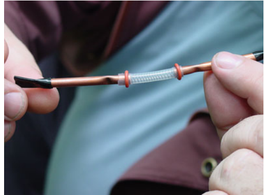
Fig. 3 A simple passive diffusion sampler. Silicone rubber tubing acts as a semipermeable membrane. After equilibration in a well or spring for 24 h, the gas inside the copper tubes is sealed with a pinch-off tool
