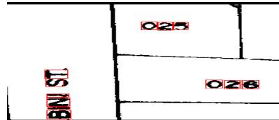
Fig. 2 It shows the detected images after processing the connected component labeling of lot numbers in the cadastral map.
