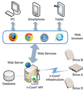
Fig. 1 The Web Services based architecture of the n-Core Polaris RTLS.
