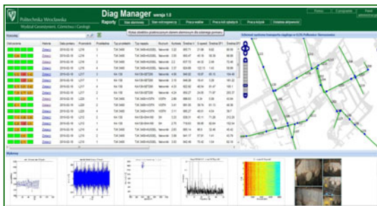
Fig 6 Main Window of Diag Manager (right: table with decisions in colours, text/numeric data, right: scheme of transportation system referenced to map of the mine, bottom – examples of signal proc. results and photo for decision validation
