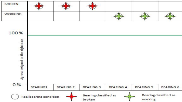
Fig. 5 Classifications of the tested bearing into broken and healthy conditions.
