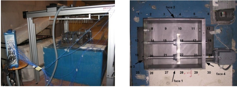
Fig. 3 Experimental Setup in a semi-anechoic room (left) Gear transmission mechanism open (right)
