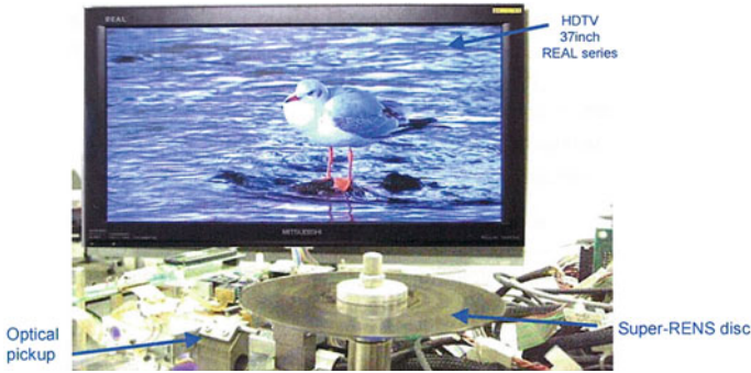
Fig. 12.15 A snapshot of a HDTV video recorded using a Super-RENS disc. Reprinted with permission by Japan Society of Applied Physics from Nakai et al. [29]
