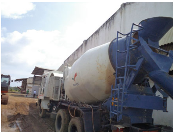
Fig. 7.11 Vehicle mounted mixer at a TSDF facility for mixing stabilisers
