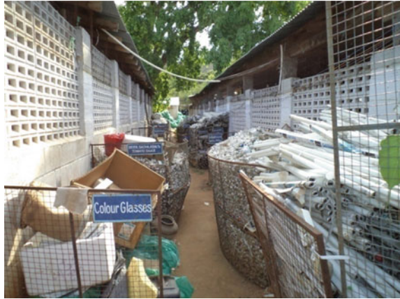
Fig. 4.3 Segregated waste at zero waste plant where components of waste are segregated to the maximum possible extent
