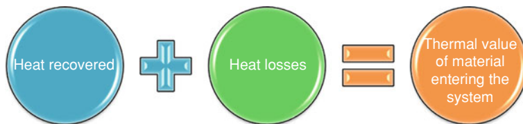
Fig. 5.18 Thermal balance in an incinerator
