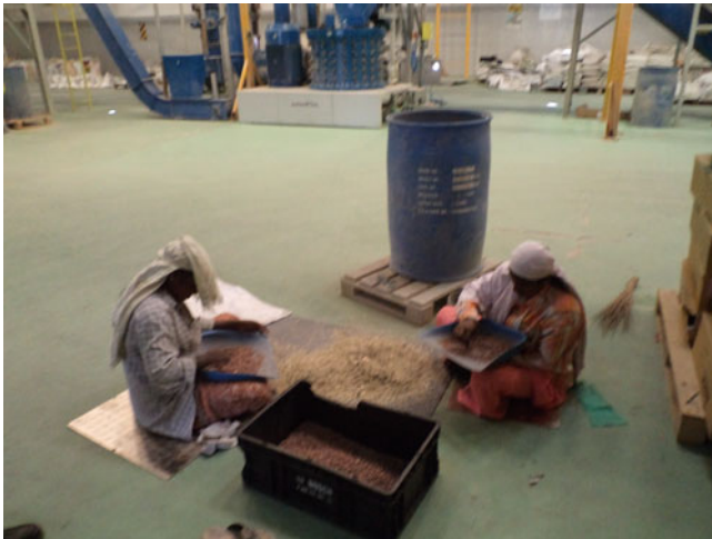
Fig. 8.11 Manual segregation of larger fraction of copper pellets and plastic after shredding and screening
