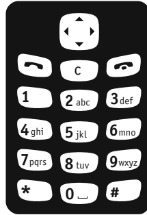
Fig. 1. The 12-key keypad of a typical Finnish mobile phone. There are three letters in the Finnish alphabet “ä”, “å” and “ö”, which are not shown on the keypad. The letters “ä” and “å” are entered pressing key “2” four times and five times respectively. The letter “ö” is entered by pressing key “6” four times.
