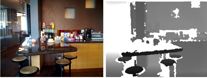
Fig. 1 (left) RGB image and (right) depth information captured by an RGB-D camera. Recent systems can capture images at a resolution of up to 640x480 pixels at 30 frames per second. White pixels in the right image have no depth value, mostly due to occlusion, max distance, relative surface angle, or surface material.
