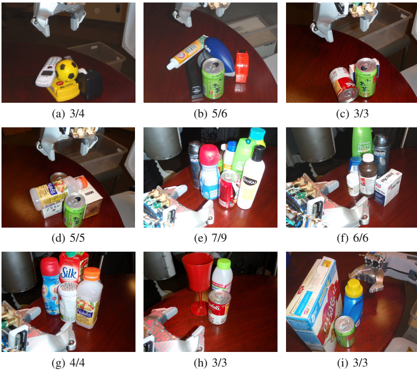
Fig. 8 A sampling of the scenes the robot attempted to clear. The fraction of objects successfully cleared from the table is noted below each picture. We attempted 7 top-grasp and 8 side-grasp scenes.
