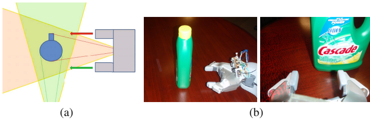
Fig. 2 (a) A view from the robot body (green cone) cannot see the protruding surface of the object. In a fairly typical planned grasp on the partial view, the gripper moves as the arrows indicate. Viewing the object from the gripper's perspective (orange cone) gives more complete data in the direction of interest. (b) An example is pictured with a large detergent bottle; the view from the front leaves significant ambiguity about the depth of the bottle, whereas the view from the gripper shows that the finger tips will not clear the object.
