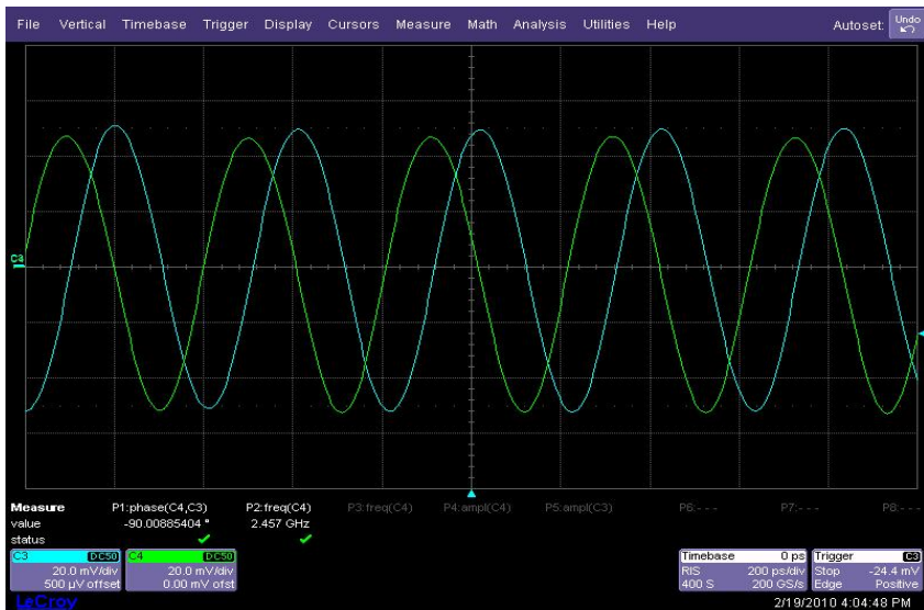
Fig. 36. Measured I/Q signal at PLL output
