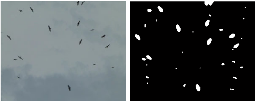
Fig. 2. Example of threshold showing the original image (left) and image after threshold (right)
