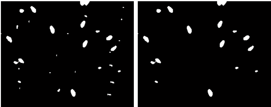
Fig. 3. Example showing before (left) and after (right) the morphological closing and opening
