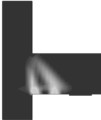
Fig. 7.82 Distribution of non-local softening parameter \kappa_2 from 3D simulations with elasto-plastic model with non-local softening ( G_c=5000 N/m, G_f=50 N/m l_c=5 mm, perfect bond) for tests of Campione et al. (2005) (Syroka et al. 2011)
