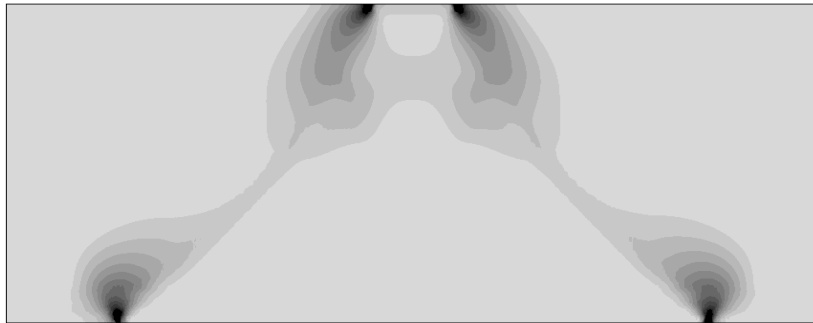
Fig. 7.37 Distribution of the non-local compressive softening parameter \bar{\kappa}_1 within elasto-plasticity for different beams at vertical displacement of u=10 mm: a) h=200 mm, b) h=400 mm, c) h=600 mm, d) h=800 mm (the beams are not appropriately scaled) (Skarżyński et al. 2010)
