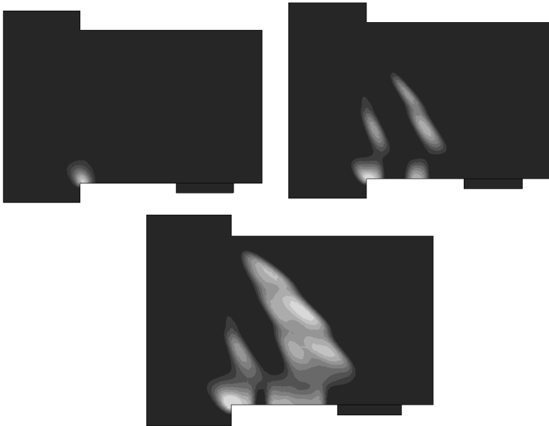
Fig. 7.85 Calculated pattern of localized zones with smeared fixed crack approach (for tests of Campione et al. 2005) (Syroka et al. 2011)
