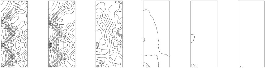
Fig. 5.15 Evolution of non-local equivalent plastic strains in the specimen during uniaxial compression (elasto-plastic model with non-local softening, three initial weak elements, m=2 , l_c=7.5 mm, \varphi=25^\circ and \psi=10^\circ ) (Bobiński and Tejchman 2004)
