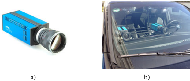
Fig. 1. Camera pco.1200 s (a) and Camera placement inside the vehicle (b).
