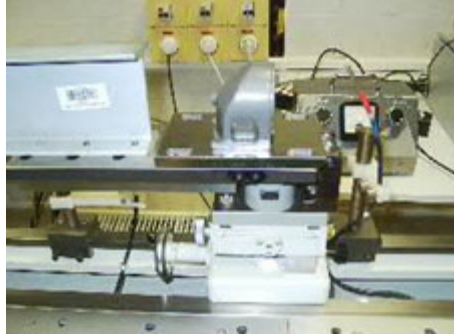
Fig. 4. Right end of the small angle generator with the autocollimator mirror.
