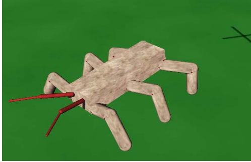
Fig. 3. Hexapod robot realised in the LpzRobots simulator. Joints between legs and thorax have two degrees of freedom and a servo motor for each axis. The joint in the middle of each leg contains only an unactuated spring.
