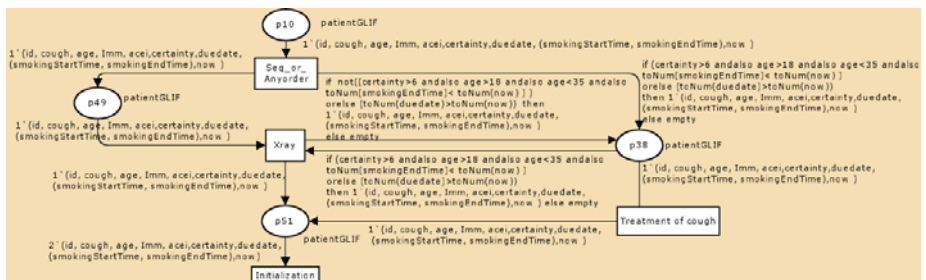
Fig. 1. Screen shot of the part of GLIF specification in CPN tools where recommendation R1) (a) iii can be checked
