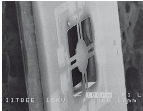
Fig. 4.6 MEMS accelerometer fabricated using polymer composite. (Source: V Ramgopal Rao, IIT Bombay)
