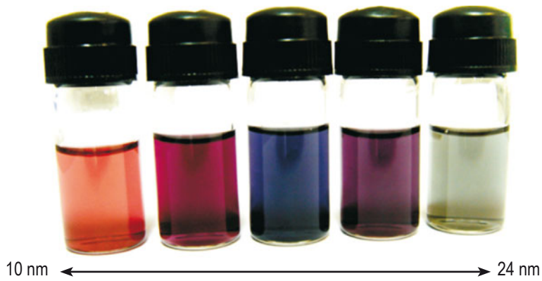
Fig. 1.5 (see page 7) Nanoshells designed to absorb various wavelengths of light – including infrared (vial at far right). (Source: http://en.wikipedia.org/wiki/File:Nano_Figure_1.png ).
