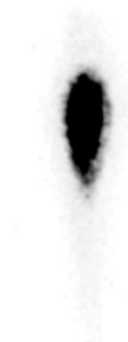
Fig. 4 TLC of sterile filtered reaction solution synthesized by the combined cationic–anionic purification method (ITLC-SG; solvent: 0.1 M citric acid)
