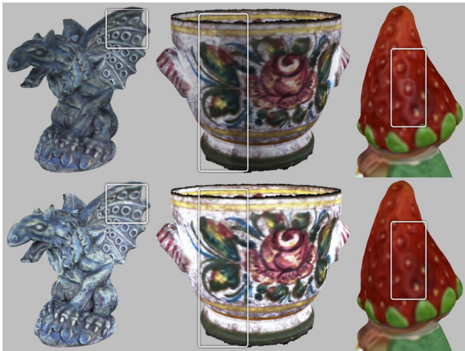
Fig. 3. Comparison of texturing obtained by a naive averaging of all input frames ( top row ) and the proposed approach using weighting masks ( bottom row )
