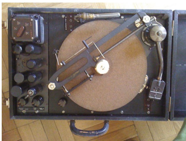
Fig. 5. Scelsi's disc-engraving recording device
