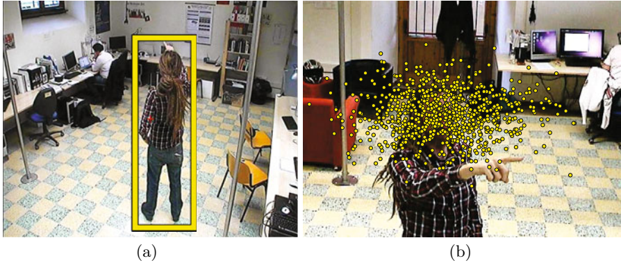
Fig. 4. Example of a frame analyzed with the proposed technique. (a): Master camera view: the target is detected by background subtraction. (b): Slave camera view: the particles show the uncertainty of the head position of the target.
