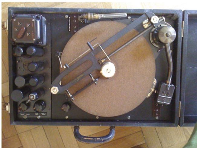
Fig. 5. Scelsi's disc-engraving recording device
