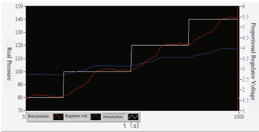
Fig. 4. Controlled common-rail pressure curve at aimed value of 80MPa , 100MPa , 120MPa , 140MPa
