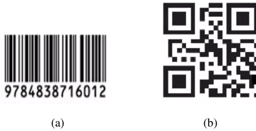
Fig. 1. One and two-dimension bar code: (a) one-dimension bar code and (b) two-dimension code
