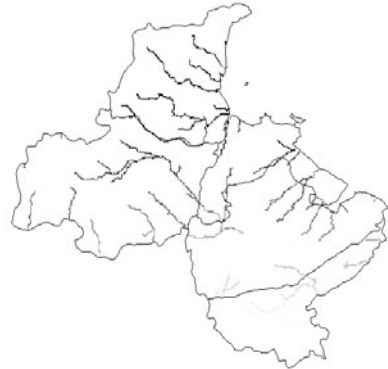
Fig. 7. River networks obtained by threshold of 5000
