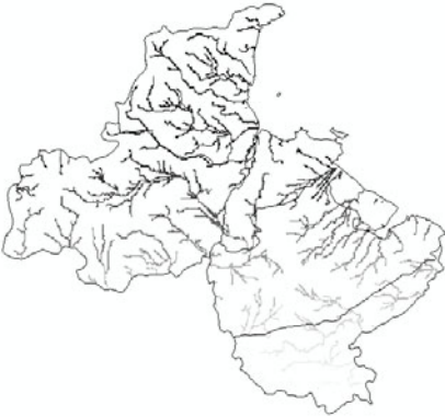
Fig. 6. River networks obtained by threshold of 1000
