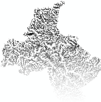
Fig. 4. River networks obtained by threshold of 90
