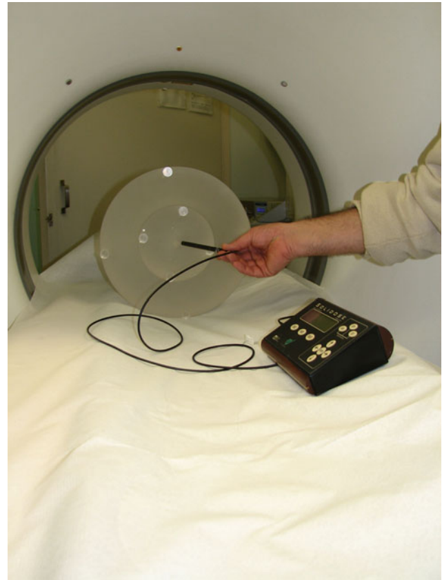
Fig. 1 Instrumentation used for CTDI determination: CTDI phantom, 10 cm long ionization chamber and electrometer
