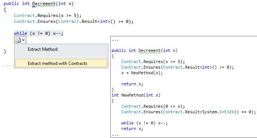
Fig. 1. A screenshot of the extract method with contracts. The suggested contract for the extracted method is correct, safe, complete and the most general one.
