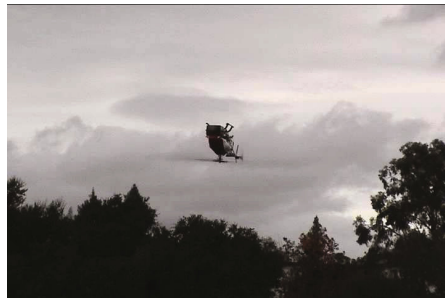
Fig. 18.4 Autonomous inverted helicopter flight (Ng et al, 2004b)(Picture reprint with permission of Andrew Ng)
