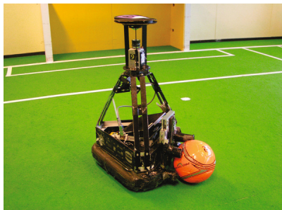
Fig. 2.6 Brainstormers MidSize league robot. The difficulty of dribbling lies in the fact, that by the rules at most one third of the ball might be covered by the robot. Not loosing the ball while turning therefore requires a sophisticated control of the robot motion.
