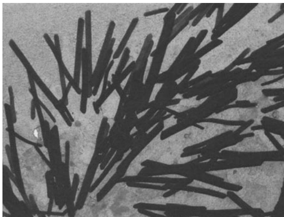
Fig. 4.5 Transmission electron micrograph of PANI nanotubes (Reproduced from [46] with the permission of Elsevier Ltd.)
