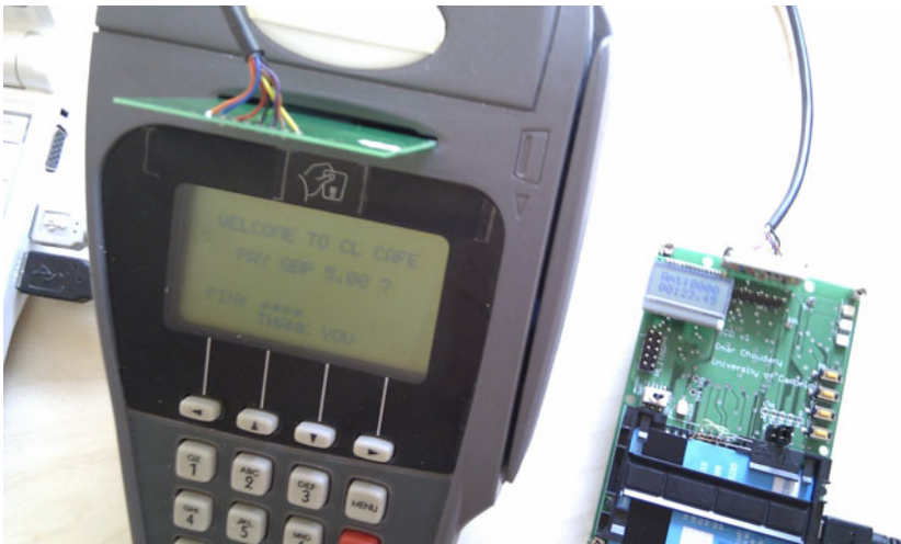
Fig. 4. Device with trusted display which can demonstrate to the customer if the protocol is being executed correctly
