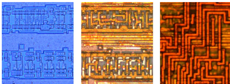
Fig. 2. Layers of a silicon chip: transistor layer, logic layer and one of the interconnect metal layers
