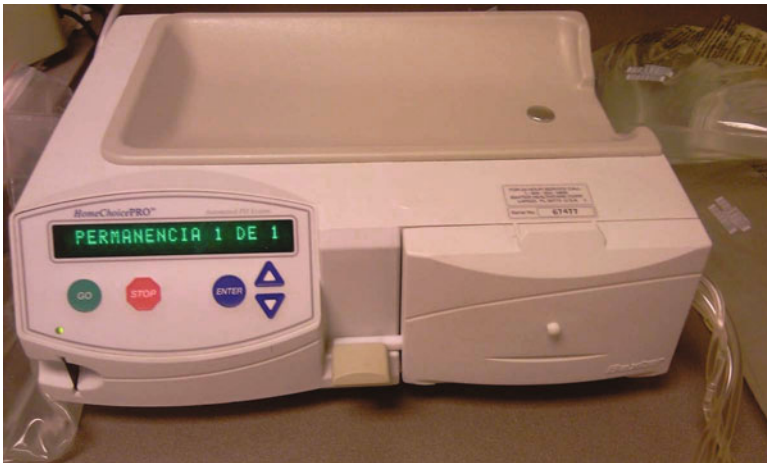
Fig. 26.1 Home Choice Pro (©Baxter Healthcare) cycler for peritoneal dialysis. The scooped surface on the top is to place the dialysate bag and the machine warms the fluid to room temperature prior to instillation in the abdominal cavity. The knob on the right hand opens a compartment to place the cassette where all the tubings are organized. The display screen on the left provides easy-to-follow instructions to patients in a variety of languages. The slit on the bottom left holds a card that records treatment data for up to 90 days and the information can either be downloaded via a modem or directly from the card onto a computer in the dialysis unit for the staff to review and advise the patient.
