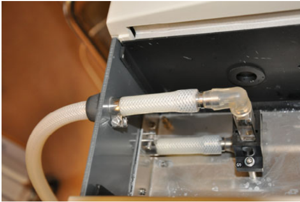
Fig. 17.7b Photo of the optical flow cuvette inserted in an UV/Vis/NIR spectrophotometer where drain tube is connected. A window for the light beam is also seen on the black wall behind the cuvette.
