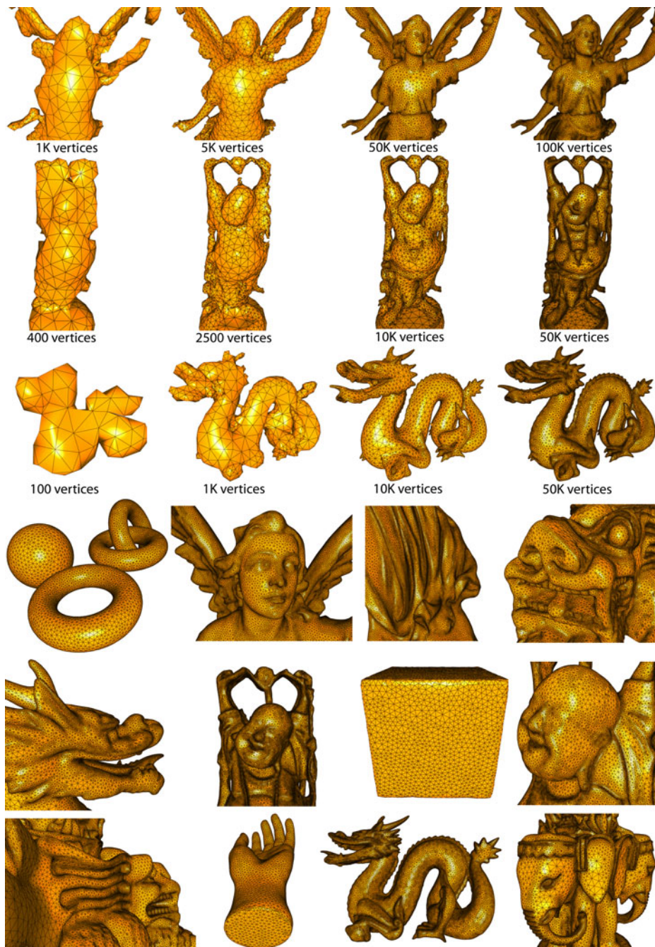
Fig. 16. Upper lines: mesh training stages with number of vertices, lower lines, assorted pictures of reconstructed models.
