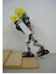
Fig. 17. A humanoid robot executing the action of climbing upstairs
