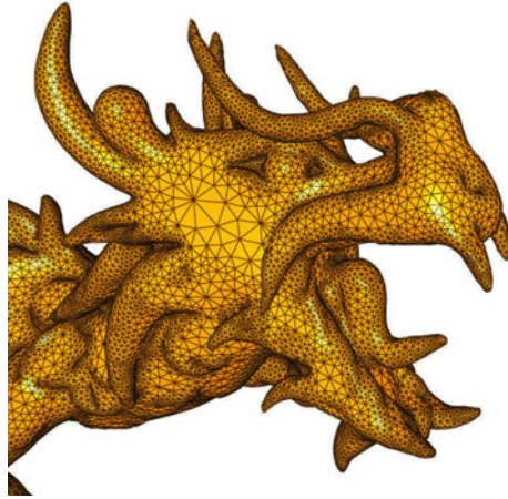
Fig. 10. Roughness adaption correlates surface curvature with mesh density, details of the model are accentuated
