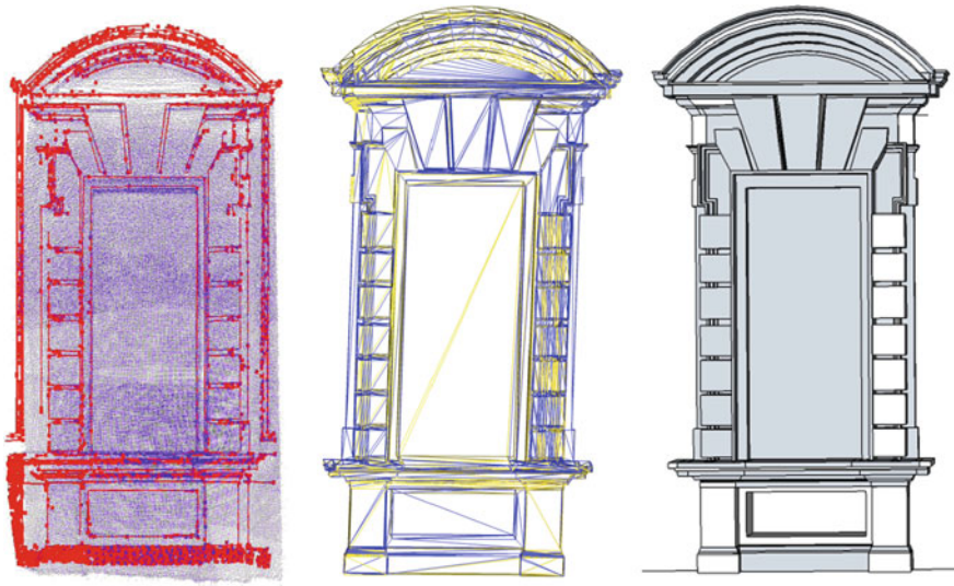
Fig. 20 TOF and break-line data integration ( left ); views of the final 3D model (wireframe visualization, centre , triangulated surface, left )
