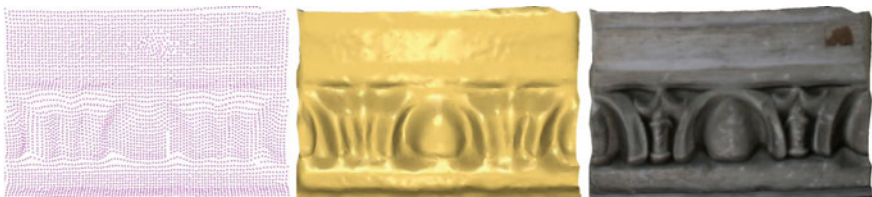
Fig. 8 Point cloud ( left ); mesh ( centre ); 3D textured model of the surveyed architectural frieze ( right )
