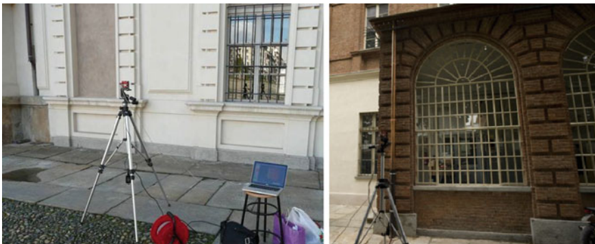
Fig. 11 TOF data acquisition of the two windows at the Valentino Castle
