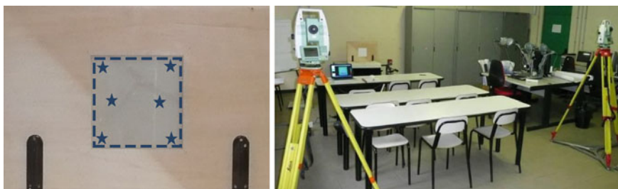
Fig. 5 Points measured for each material in order to estimate the spatial position ( left ); Topographic measurements for the estimation of the camera and tested object positions ( right )
