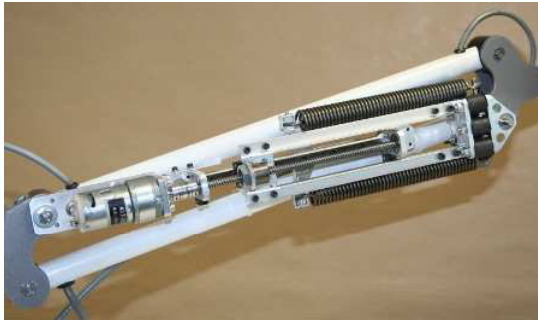
Fig. 3. Linear actuator with tension springs
