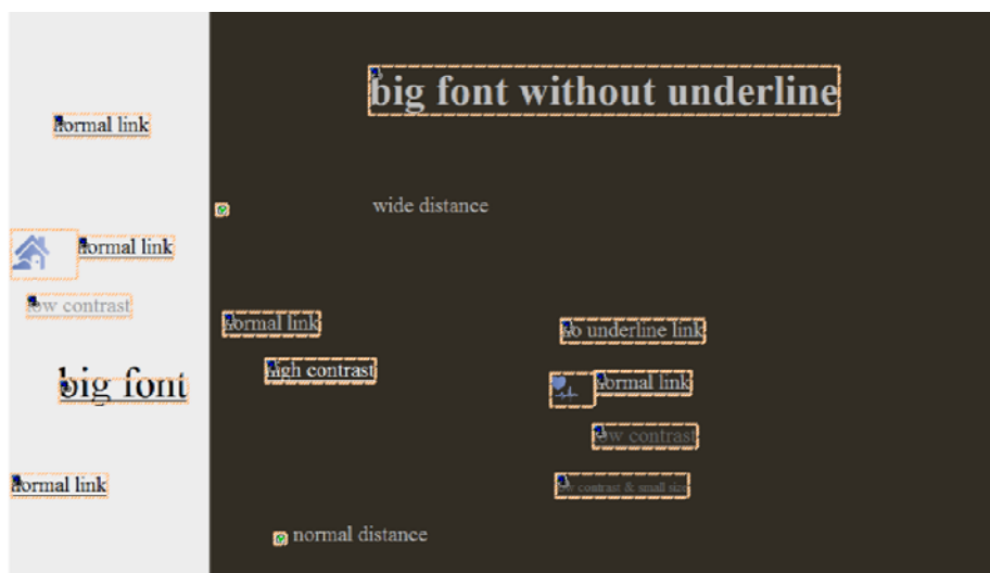
Fig. 3. Automatically imported UI model of a web page with annotated locations for GUI elements (hyperlinks, icons, checkboxes)
