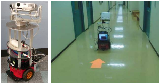
Fig. 1. A photo of the ubiquitous display system on a wheeled robot (left) and its application marking an arrow on the floor for supporting navigation (right). Source: Lee (2007)
