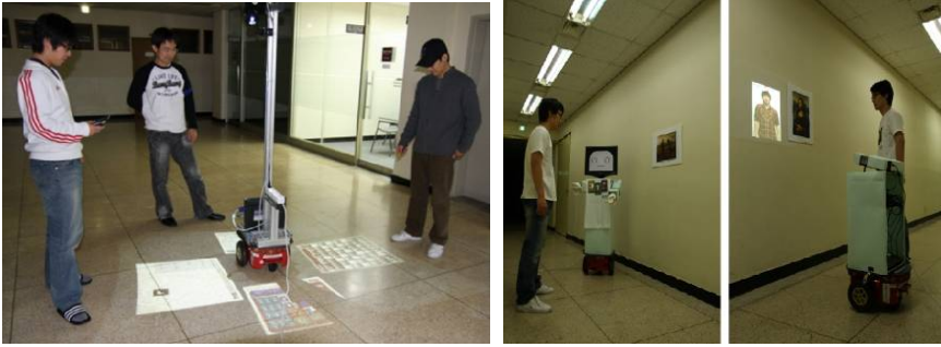
Fig. 2. Left: A proposed HRI platform with floor projection, Park et al. (2009). Middle and right: Museums guidance by (near) humanoid robot (middle) and by the projector robot (right), Kwon et al. (2010).
