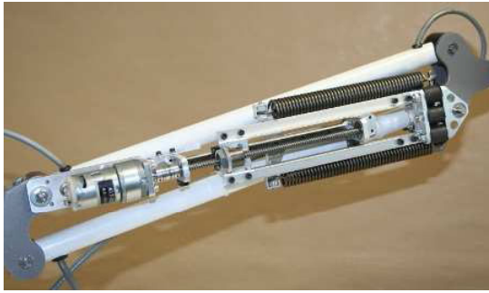
Fig. 3. Linear actuator with tension springs
