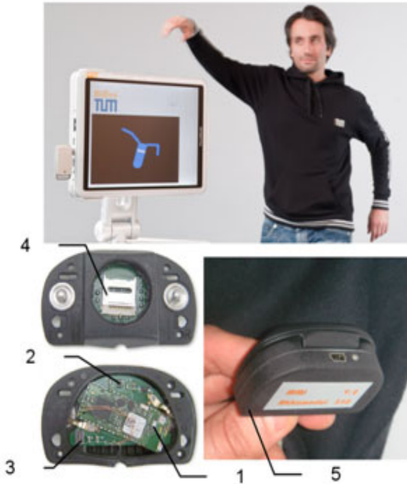
Fig. 2. Above: Pullover being used. Below, left side: electronics unit. Below, right side: battery
