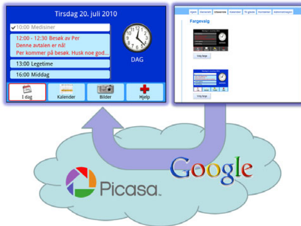
Fig. 1. Mylife services presented on primary end-user's device (upper left). Secondary end-user's web for configuration and administration (upper right), including personalisation (appearance and choice of services), and feeding in content, e.g. appointments/reminders to calendar, or photos to album(s).
