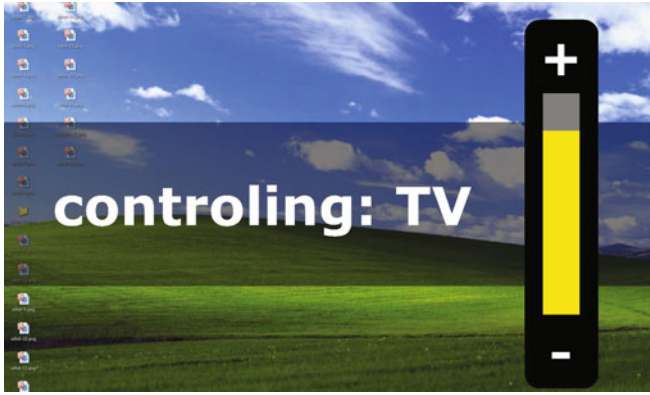
Fig. 5. Controlling a device by moving the hand vertically to set a level, e.g. the volume of a TV
