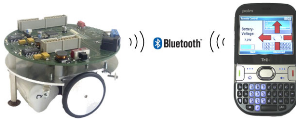
Fig. 5 Remote control and wireless debugging via Bluetooth
