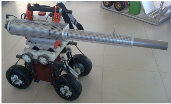
Fig. 3 Germán LaRA with a thermonebulizer for Greenhouse fumigation.
