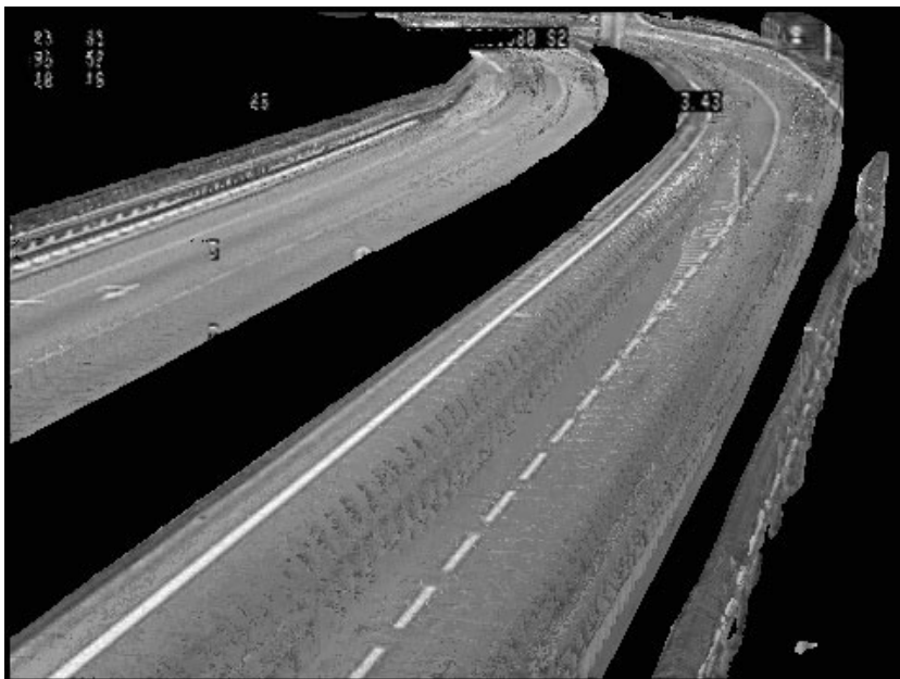
Fig. 5 Provable background image quantized with 64 gray level values.
