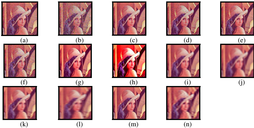
Fig. 1. Reference image simulated with different types of distortion. (a), (b) Salt & Pepper noise. (c), (d) Speckle noise. (e), (f) Gaussian noise. (g), (h) Contrast stretching. (i), (j) Gaussian blurring. (k), (l) Motion blurring. (m), (n) Compression.
