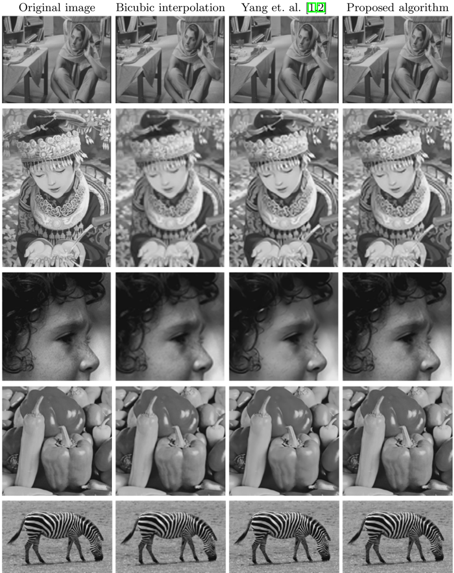
Fig. 5. Visual comparison: Portions from various images (from top to bottom: barbara , comic , face , pepper , zebra ). Left to right: the original image, bicubic interpolation, Yang et. al. [12] and the proposed algorithm (using the more complex method for dictionary update). Note that the proposed algorithm produces sharper results, preserves the small details of the image and has less visual artifacts compared with bicubic interpolation and Yang et. al. [12].
