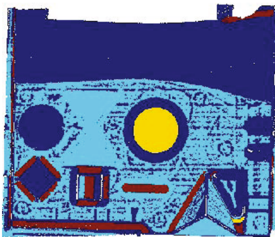
Fig. 15. Model selection (dark blue: no model; cyan: plane; yellow: sphere; red: cylinder)
