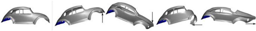
Fig. 8. Beetle Car Deformations. The original beetle model (left) is deformed by fixing the rear of the car and moving the handle at the engine hood into four different directions (right).
