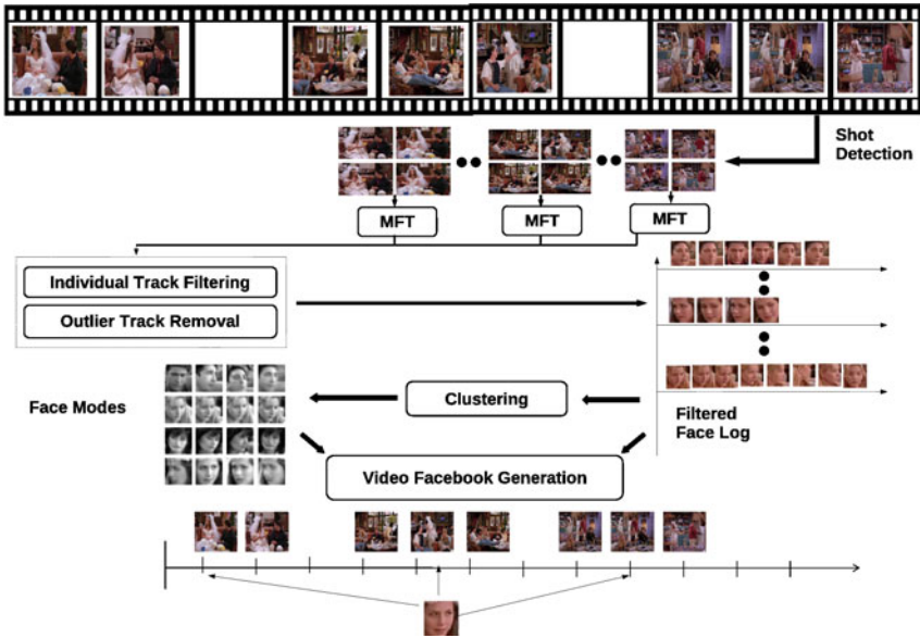
Fig. 1. The shot segmented input video is subjected to multiple face tracking (Section 2) to extract face tracks from individual shots, which are filtered in two stages to remove outliers (Section 3). The resulting face log is clustered using a GMM variant to discover the modes of facial appearances of different people in varying facial poses. The face based video index is generated by analyzing the track and cluster correspondences, which we call the Video Face Book .
