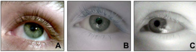
Fig. 2. Image of the human eye, from left: image captured by a regular web-camera, without the infrared light blocking filter, and with visible light blocking filter (with a fragment of the burned analog camera film). Notice that the dark pupil is very clearly visible in the rightmost image.
