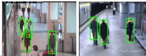
Fig. 8. Results of Pedestrian detection. Yellow-contour model is the best hypothesis for the hierarchy models.
