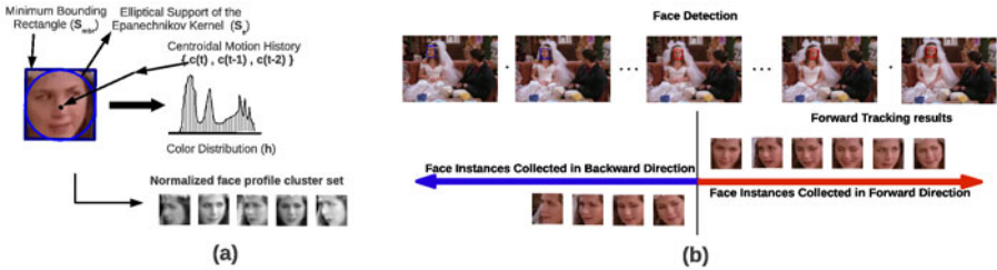
Fig. 2. (a) Color distribution \mathbf{H}(F) , second order motion model and the normalized face cluster set ( \mathbf{NFCS}(F) ) are used for face representation and tracking . (b) Backward-Forward tracking – Jennifer Aniston’s face gets detected somewhere at the middle of the shot interval; multiple face tracker detects a new face region and starts tracking (marked with red bounding box) in forward direction. Mean-shift tracker initialized from the first detection is used to localize the face in backward direction (marked with blue bounding box).
