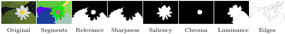
Fig. 2. Spring lily pads , by jseyerle; its segmentation map; its 5 different contrasting regions binary maps –each with two regions, with white being the regions above the threshold, and black the regions below the threshold – and its edge map
