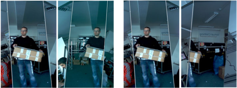
Fig. 9. Stereo content captured by 3D-OMNICAM: left and right view from regular stereo pair at same mirror segment (left) and stereo content from virtual stereo pair across neighbored mirror segments (right)
