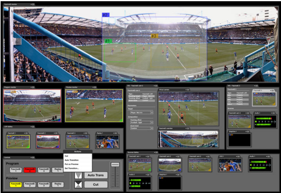
Fig. 3. Sketch of the EditorUI interface. The upper part renders the whole panorama and displays views that are defined by the PSE as color overlay boxes.
