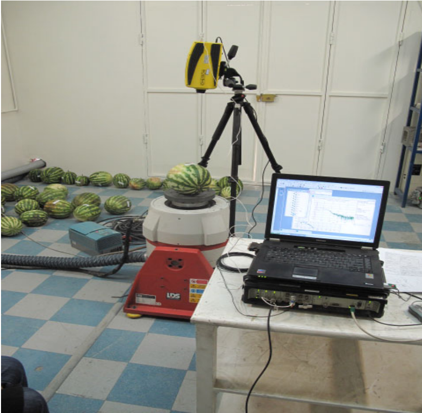
Fig. 2. LDV sensed response of the fruit in upper surface as output signal
