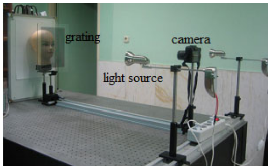
Fig. 4. Experimental arrangement in shadow Moiré technique
