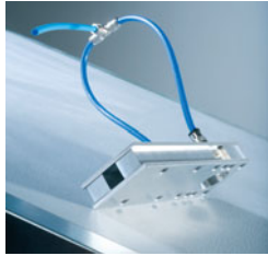
Fig. 7. The Coanda gripper: Prototype [16]
