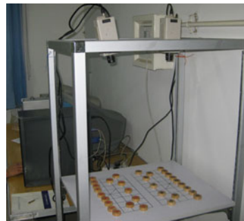
Fig. 2. Prototype of a machine vision system
