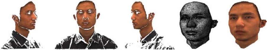
Fig. 2a. The point cloud data
