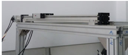
Fig. 1. The experimental platform of 2-DOF Gantry Crane Robot
