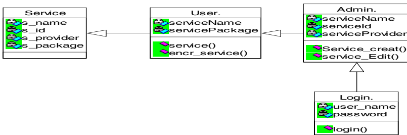
Fig. 1. Class Diagram for Web Services Application Design
