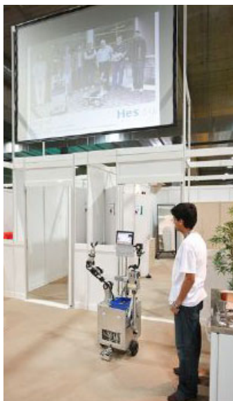
Fig. 7. General view of RH4-Y robot in Graz during the “Introduce” test, where the robot autonomously enters home, moves to the living room, talks, presenting itself and team, then leaves
