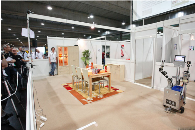
Fig. 6. Our robot line of service robots in a domestic context, RH-Y (here, RH4-Y in Robocup world competition, in Graz, Austria, 2009) consists of complex systems, featuring classical controllers (PLC, elaborated servo-controllers), computer and processors (tablet PC, etc.) and software solutions (Windows, Linux), as well as novel components, such as our multi-agent, real-time and simulation environment (Piaget), multiple cognitive capabilities such as sensing distances in 3D, recognizing scenes, gestures and speech, locating objects, learning new tasks and topologies, and generating coordinated motions and trajectories as well as producing their own speech and graphics, following humans and handling objects (Re. [3] and numerous videos at http://rahe.populus.ch )
